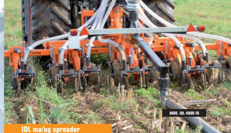
Allows the injection of slurry (digestion or manure) to a maximum depth of 15 cm. The system was designed to be used in areas where significant crop residues are present.
